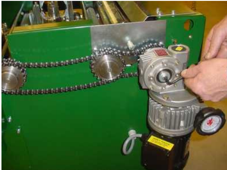
To remove the feed motor, pick up on it and rock it off the rubber feed roller shaft.
