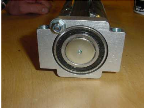
The Bearing back in place.
