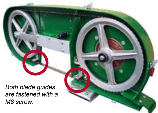
*Both blade guides are fastened with a M8 screw.*
