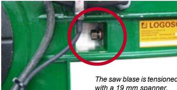
*The saw blade is tensioned with a 19 mm spanner.*
