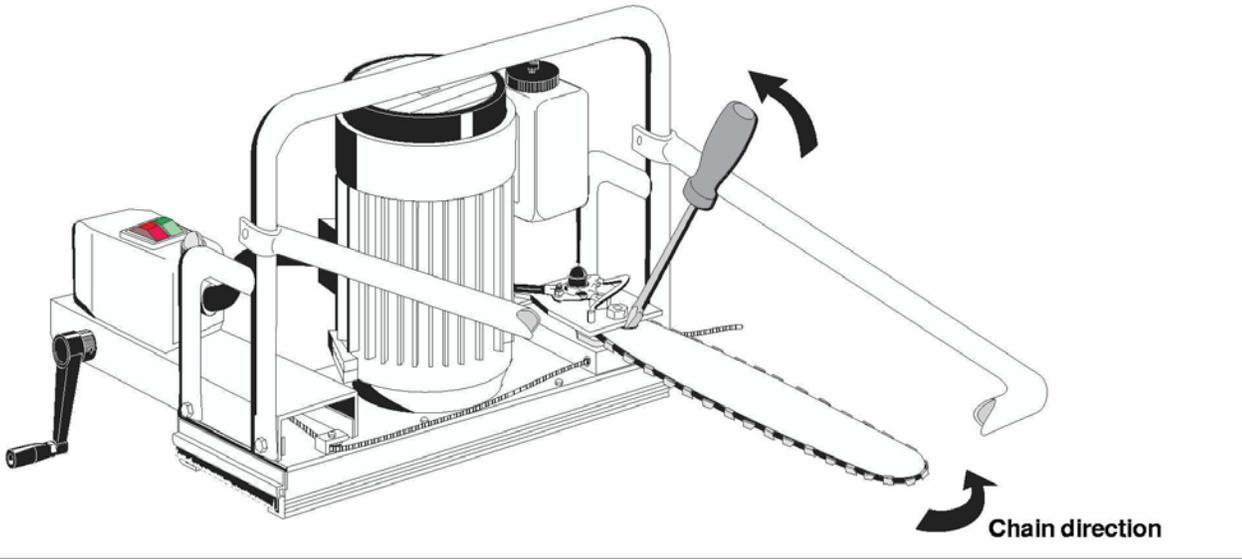
First check that the unit is unplugged. Then remove the bar nuts and the bar plate. Fit the bar and chain and return the bar plate to its place.
