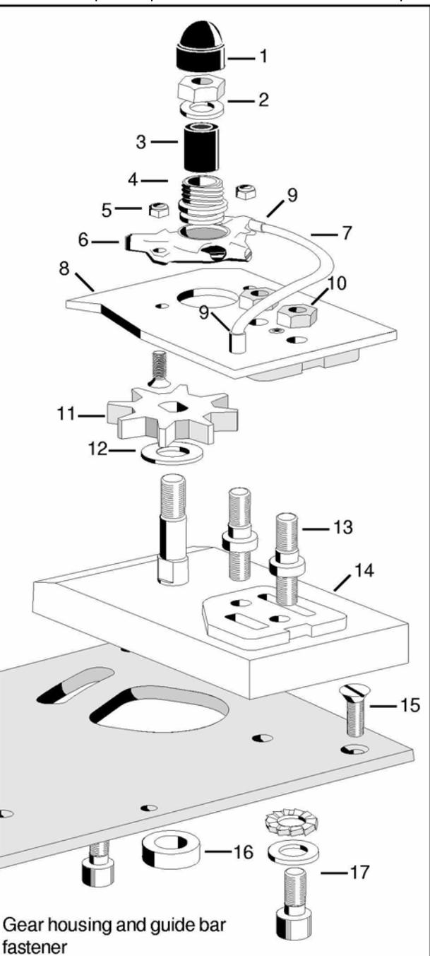
Gear housing and guide bar fastener
