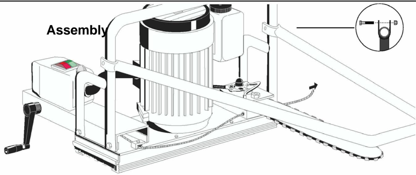
Fit the control arm to the electric saw using four M6x20 bolts and nuts. First loosen the protective yoke. Then place the control arm in position and push two bolts through the protective yoke, the control arm and its mount, tightening the nut on the inside. Use two more bolts to fasten the other side of the control arm. To tighten, use two 10 mm cap keys.
