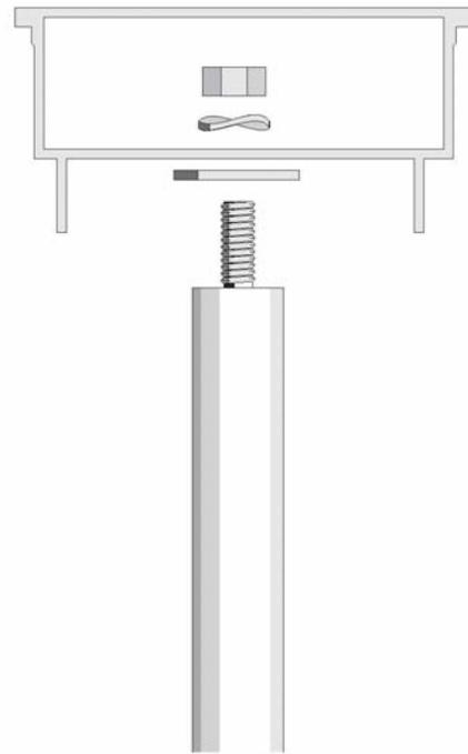
Fit the support legs to the ends of the saw mill guide rail as shown above. If the ground is loose, the saw mill and the struts ought to be attached to a wooden frame in order not to sink into the earth.
